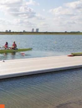
System Olympia has been specially developed by Inter Boat Marinas for (professional) rowing. The system is optimally customised for use by rowers and canoeists and is also very suitable for use as a fishing pier or floating terrace. The pontoon has a special low freeboard of 15 cm, high buoyancy, a rounded side and anti-slip deck material that is friendly to the oars.
